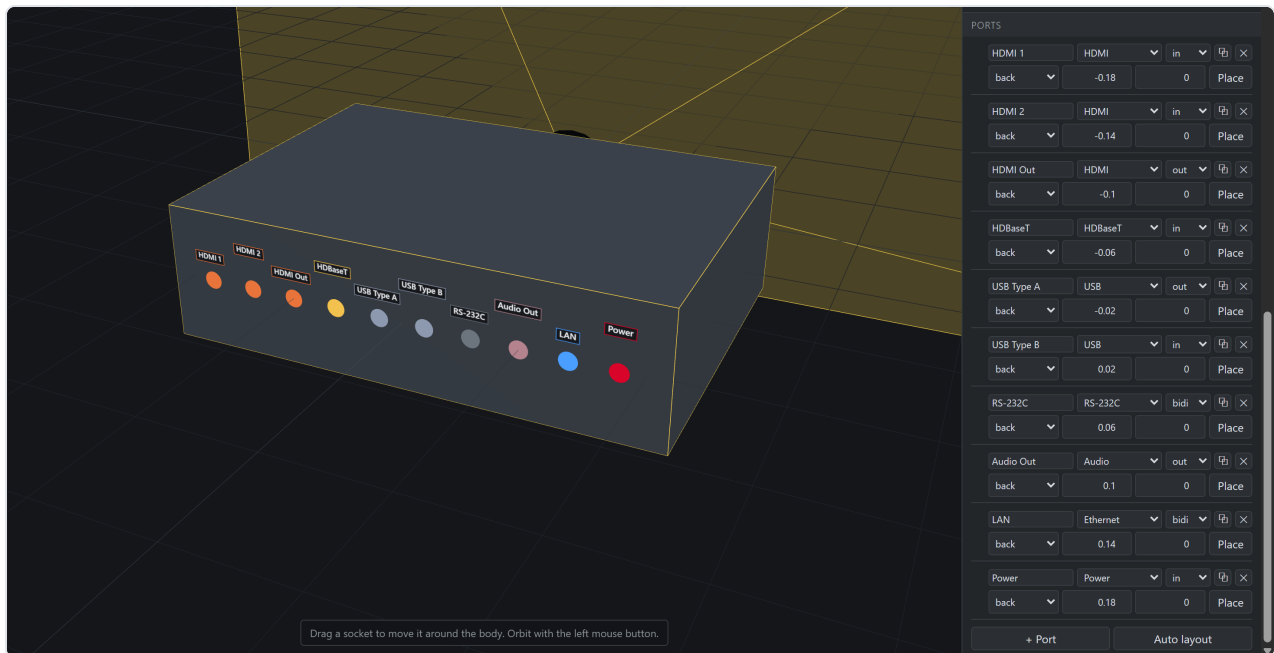
Figure 7.4 The EB-L695SE's panel in both the places it exists: ten sockets on the machine's own back face, and the rows that put them there. Each row takes two lines — a name, its type and its direction, then the face it sits on and its offset across and up from that face's centre. The two are one thing seen twice: drag a socket on the body and the numbers follow it , " Place " arms a click for putting one down by pointing, and "☰" duplicates a socket beside its twin — which is how a row of four HDMI's gets built. The preview opens on the machine's front; this is it orbited round to the back, where this projector keeps everything.
